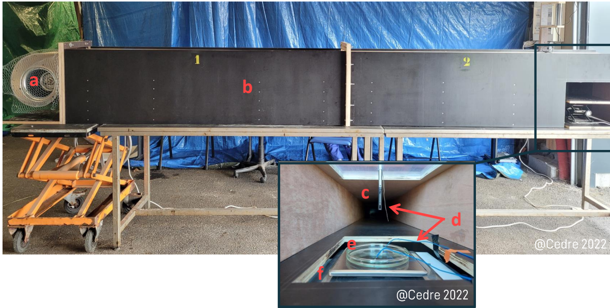
Figure c. Wide shot of the wind tunnel with a zoomed-in image of the petri dish and the operating sensors inside the gallery (temperature probes and anemometer): a) fan; b) tunnel; c) anemometer; d) thermocouples ; e) petri-dish and f) weighing scale.
