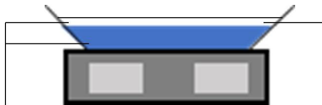
Figure 38. Scheme of the scale with suited holes to place temperature probes, two on the surface and one at the bottom.
