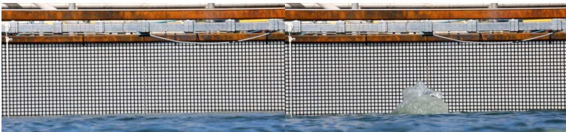
Figure 8 : Example of seawater free surface elevation observed during a methane gas release in the bottom of seawater pool (video 972A2545 - Flow rate \text{CH}_4 Q_v = 100 \text{ l/min} )
