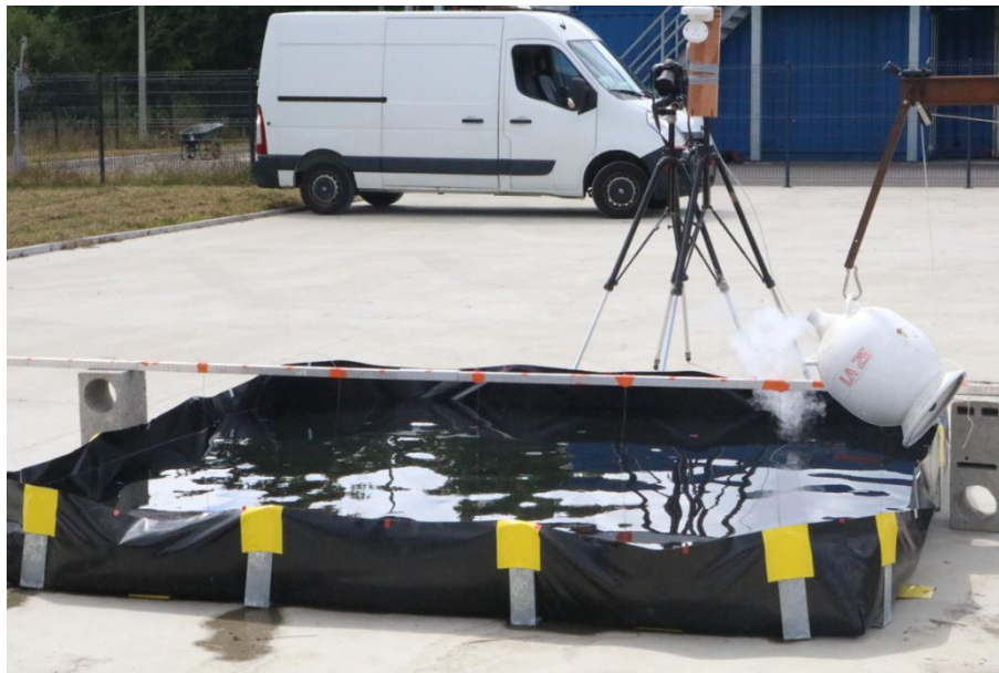
Figure 41: Temporal Photograph of the experimental setup prior to the cryogenic nitrogen release. The portable water pool is filled with seawater. The open-top cryogenic nitrogen vessel is visible in its initial tilted position at the edge of the pool, held by the wire-and-pulley release mechanism. The thermocouple support rail is mounted along the central axis of the pool.
