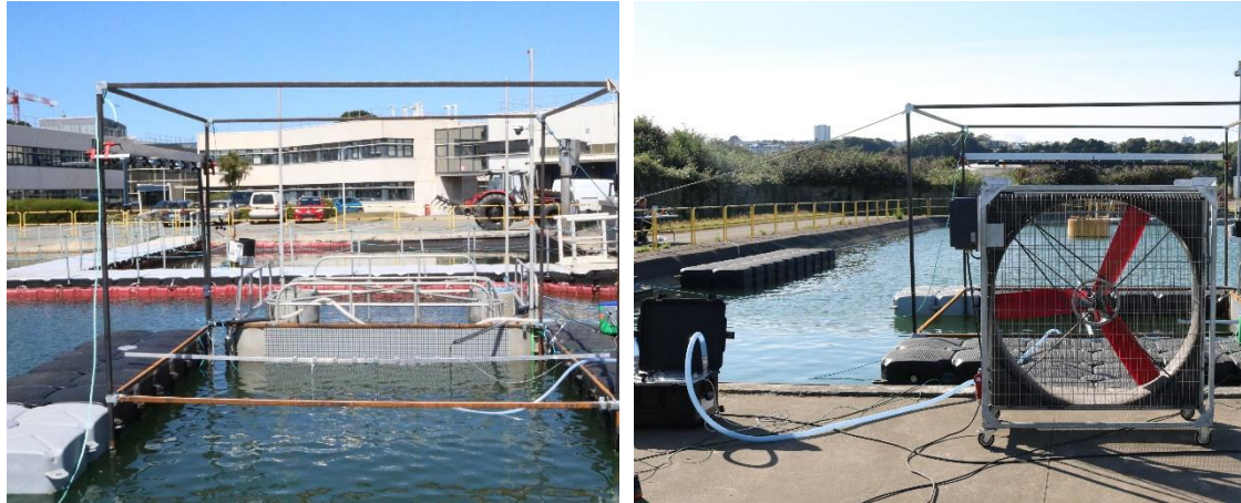
Figure 16: Front view (left image) and lateral side view of the CH_4 gas release experimental setup (right image).
