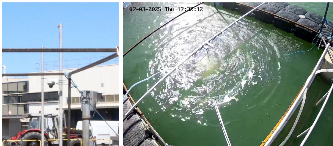
Figure 17: Zoom on the surveillance dome camera (left image) and the observed scene of the seawater free surface variation resulting from the CH_4 gas release at a flow rate Q_v of 100 l/min (right image)
