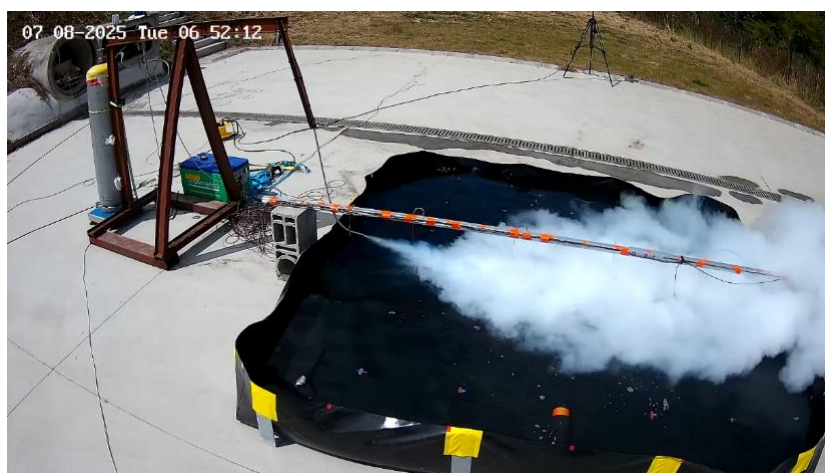
Figure 33: Aerial view of the pressurized liquid ammonia release onto the water surface, recorded by the surveillance camera during the test. A dense white plume, characteristic of a two-phase mixture generated by the adiabatic expansion of liquid ammonia at the nozzle exit, propagates along the thermocouple array axis, ensuring direct exposure of both air and water sensors to the ammonia cloud.
