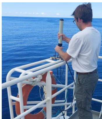
Figure 7: setting up goniometer to localise the CLS buoys dropped at sea.
